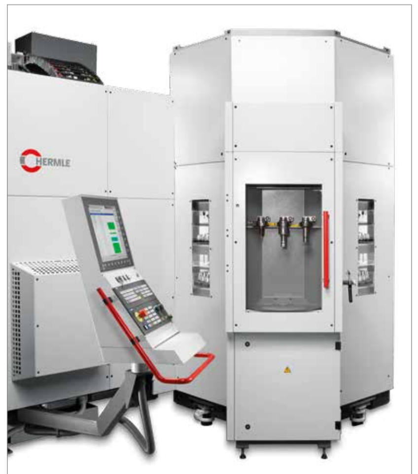
Configuration for the C 32 and C 42 / MT. Machine control panel can be swiveled to the loading and unloading position
