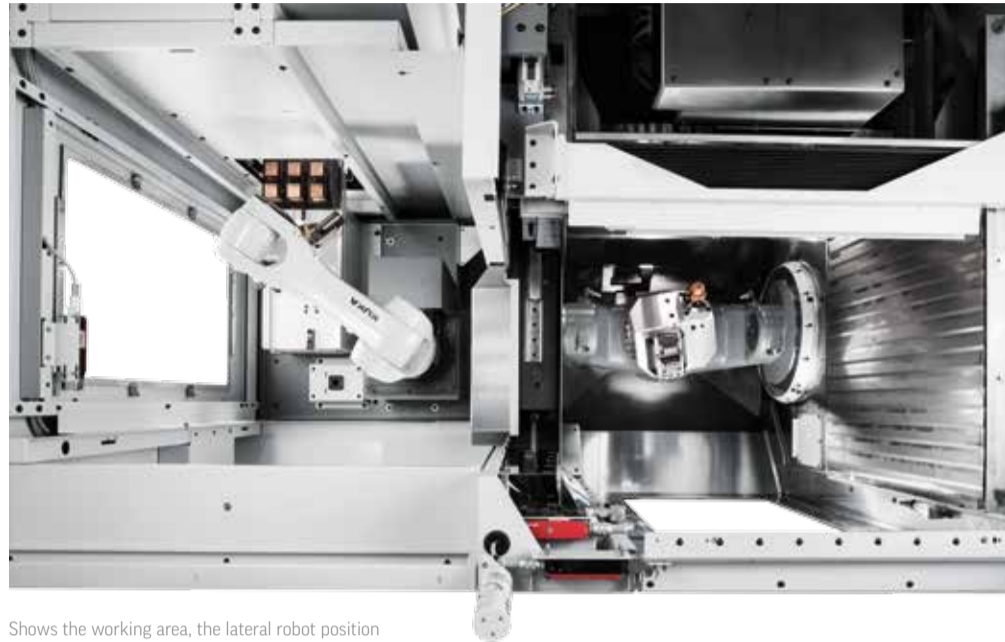
Shows the working area, the lateral robot position with die during the change process (from above)
