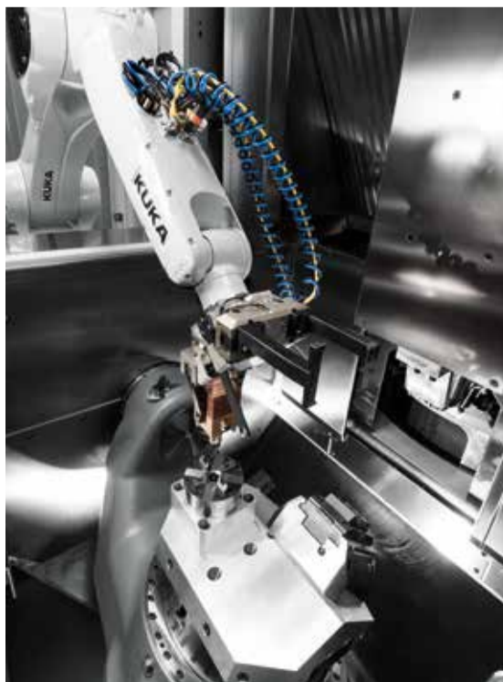
shows the compact working area of the C 12 U when loading a workpiece using the RS 05 robot system
