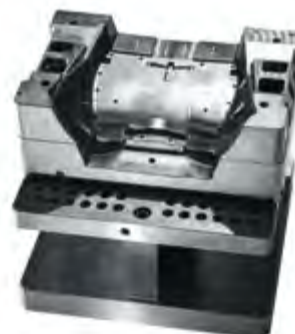
Picture shows a mould insert made of 1.2767/56HRC for which, after 5-axis simultaneous milling with very small cutters (D0.6), only a few electrodes were necessary for spark eroding
