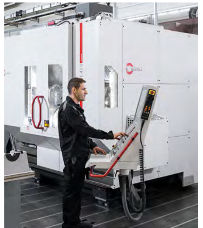
The C 42 U dynamic 5-axis CNC high-power machining centre installed at CERN's MME department, equipped with precision packages I and II for highly precise, reproducibly exact quality machining within tolerances of \pm 0.5 \mu\text{m}
