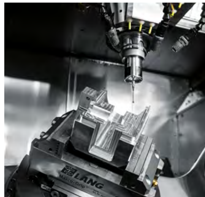
Picture shows the working range of the high-performance, 5-axis CNC machining centre C 32 U with an NC rotary table for 5-axis/5-sided complete/simultaneous machining in one setup
