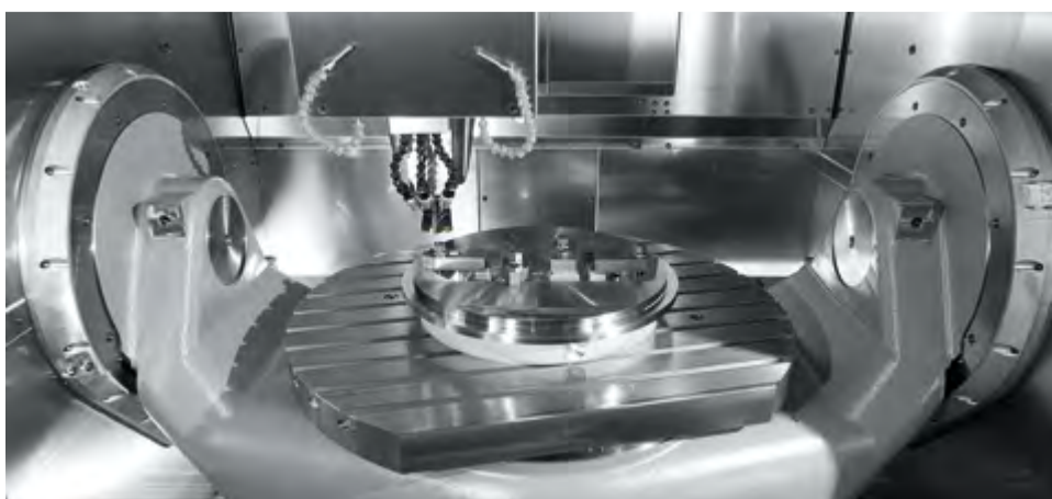
Image shows the generous working area of the C 42 U machining centre with the NC swivelling rotary table of diameter 800 x 630 mm (axes A and C) used for 5-axis/5-side complete and simultaneous machining of diverse components for particle accelerators
