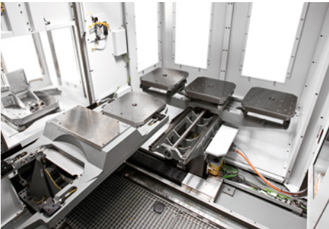
Pallet changer PW 850 with storage
