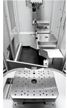
Pallet storage from the pallet changer PW 150
